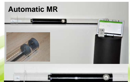
Fig. 2 Automatic UHD MR camera modules for concurrent imaging by one operator in large 'rhizotrons' facilities
